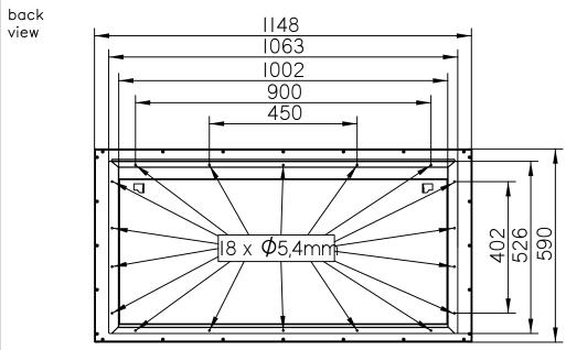
The installation box must be fastened with the correct fastening material.
